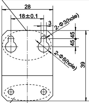
Holes for attaching to the U-WAVE-R (2 pieces)
