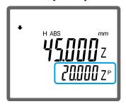
The difference with the previous measurement can be checked simply by reading the value displayed in the bottom row.
